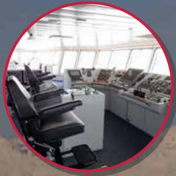
Integrated Alarm Monitoring Control Systems (IAMCS)
